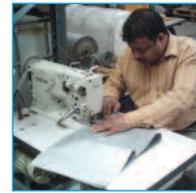
ContraFlex® is manufactured in the form of a jacket, usually 61mm thick. The thickness of the jacket can vary to suit the requirements of the application and duties. Manufacture can be undertaken either at our facilities or, where appropriate, at the project site.
