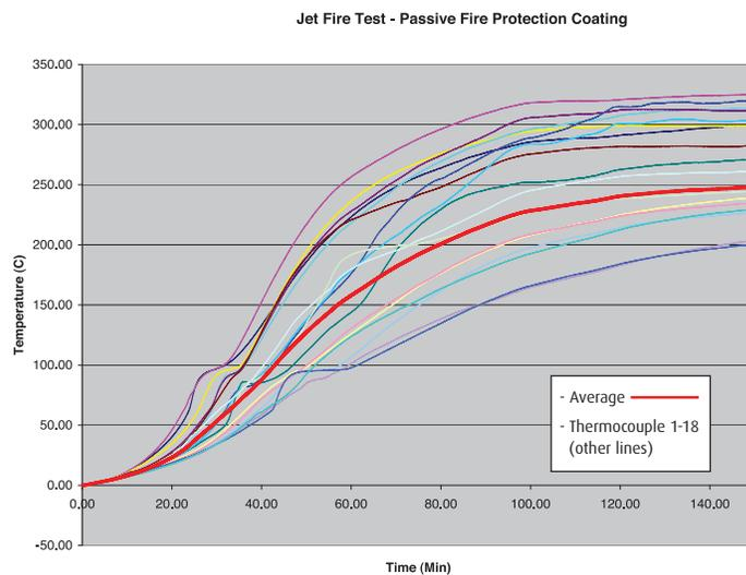
The very low temperature rise associated with ContraFlame® JF120 system makes possible operating temperatures as high as 185°C whilst still assuring safe substrate temperature during the jet fire.
